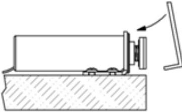
Insert the latch in the lock after prior centering the latch bar and fitting the alignment piece 3 over the bar (see section 3).
