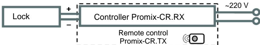
**Provide a reliable electriccontact. To prevent short-circuit, insulate places of connection.**
