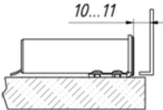
Mount the lock on an immobile surface. The distance between the inner surface of the closed door to the lock nut must be 10-11 mm, which guarantees the necessary free movement of the door within 3-4 mm with the lock closed. Connect the lock in accordance with 6.2.
