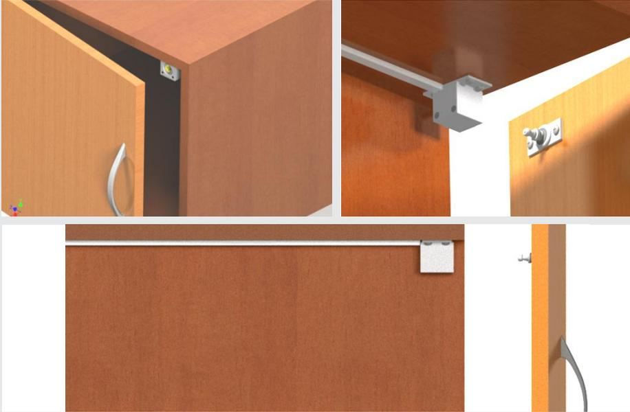
**Example of the lock mounting on a sliding door (rolling door cabinet).**
